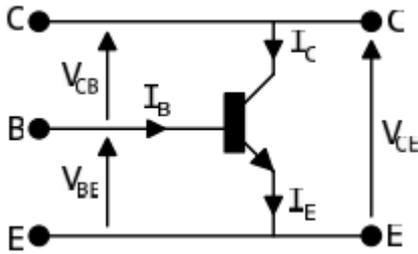
$$\begin{cases} V_{CE} = V_{CB} + V_{BE} \\ I_E = I_C + I_B \\ I_C = \beta I_B \end{cases}$$
